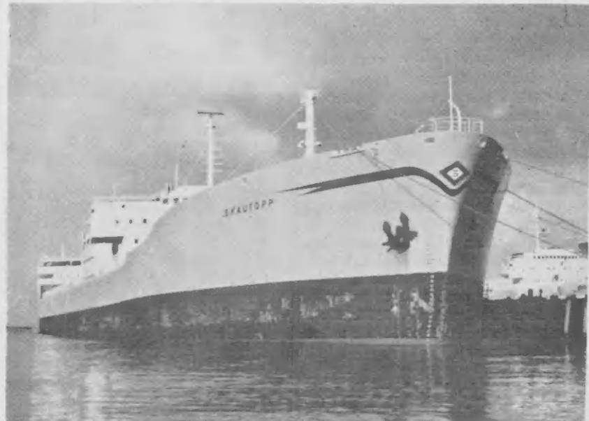
THE SKAUTOPP'S 19,000 horsepower diesel enables it to cruise at speeds up to 15.7 knots at 110 revolutions a minute. E DIESEL di 19,000 forza di cabai di Skautopp ta permitie'le cruza na velocidad te 15.7 milla na 110 revolucion pa minuut.
